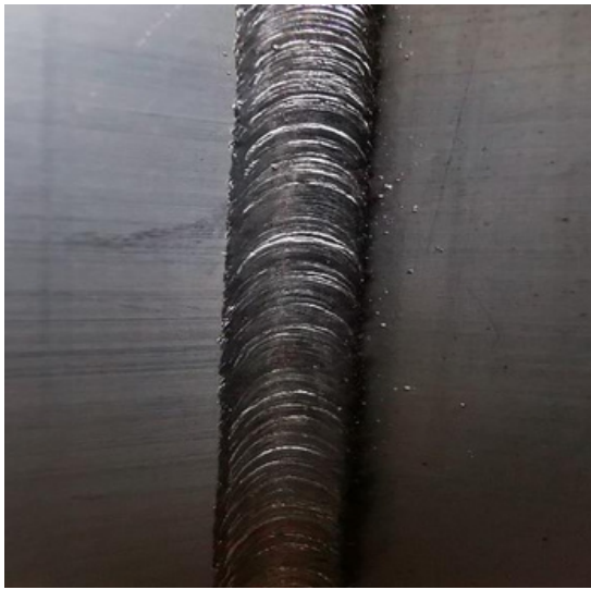
2.0mm Fillet Weld 1.2mm 5356 wire
