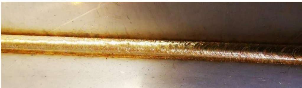
2.0mm Stainless Steel. 1.2mm Fillet Weld, 1.0mm 316L filler wire
