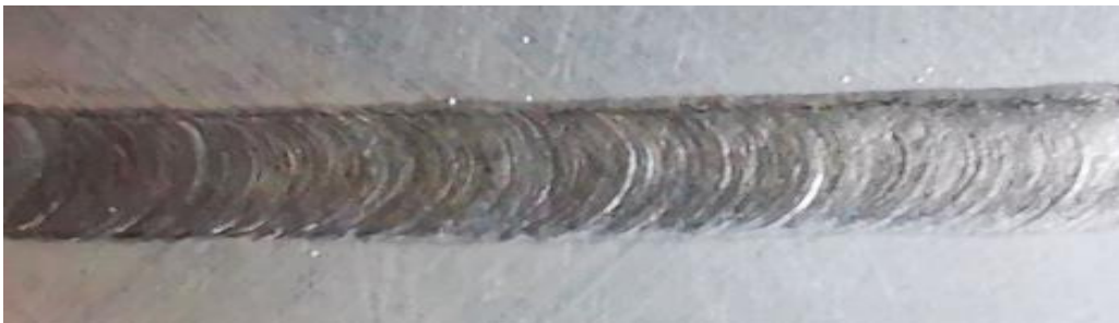
2.0mm Aluminium, Butt Weld. 1.2mm 5356 wire
