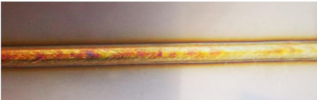
2.0mm Stainless Steel. Butt weld 1.0mm gap, 1.0mm 316L filler wire
